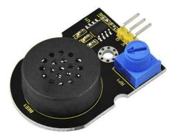
We can turn the potentiometer to adjust the sound amplification, that is, to adjust the sound volume.
