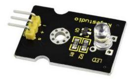
There are three lead-out pins on the module, respectively negative pin(marked -), positive pin(marked +) and signal pin(marked S).
