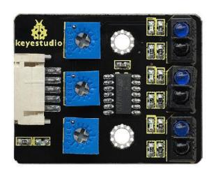
During the process of detection, black is active at HIGH level, but white is active at LOW. The detection height is 0-3 cm.
