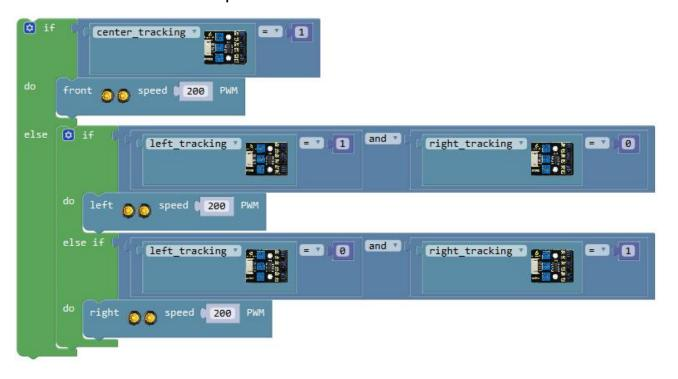
In the case that the center tracking sensor detects white line, if the left tracking sensor detects white line and the right tracking sensor detects white line, the robot will stop running; if the left tracking sensor detects black line and the right tracking sensor detects black line, the robot will stop running.
