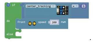
Next, go to the "Logic", drag out the block from the "Desktop\_Car\_V3" into the first input box at the left side of "="; drag the Math" into the
