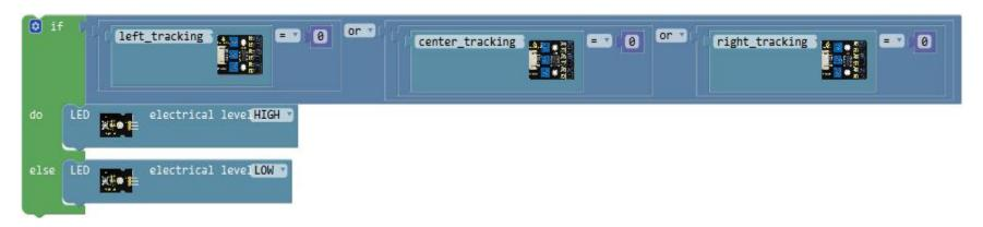
Now we have written the code of tracking sensor controlling white LED module. Upload the complete to see the final result!
