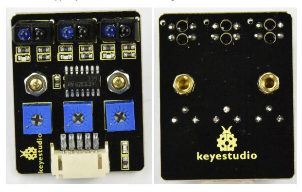
After that, mount the line tracking sensor on the Acrylic board with two M3\*6MM round-head screws. Tighten the
