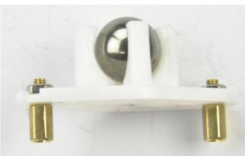
Screw the W420 ball caster wheel on the Acrylic bottom board with two M3\*6MM round-head screws, two M3 Nuts, two M3\*8+6MM single-pass copper pillars. Tighten the screws with a screwdriver.
