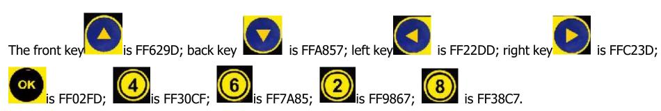
As the command key of IR remote control is hexadecimal code, the front must add 0x.
