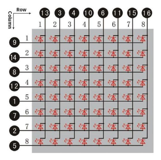
For instance, to light up the LED on row 1 and column 1, increase the voltage of pin 9 and reduce the voltage of pin 13.
