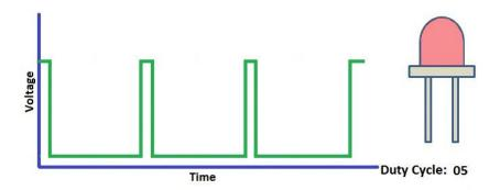
For the Arduino digital port voltage output, there are only LOW and HIGH, which correspond to the voltage output of 0V and 5V. You can define LOW as 0 and HIGH as 1, and let the Arduino output five hundred 0 or 1 signals within 1 second.
