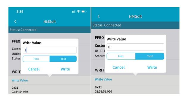
Click "Write" on APP, when you enter 1, LED will be on, when you input 0, LED will be off. (Remember to remove the Bluetooth module after finishing
