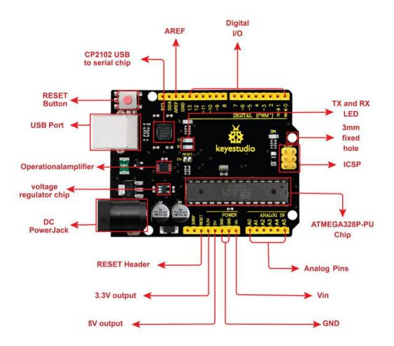
It has 14 digital input/output pins (of which 6 can be used as PWM output s), 6 analog inputs, a 16 MHz quartz crystal, a USB connection, a power jack, 2 ICSP headers and a reset button.
