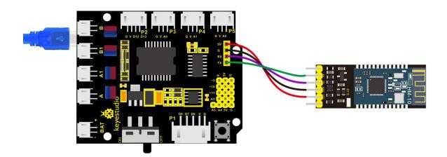
Pay attention to the pin direction when inserting Bluetooth module, and don't insert it before uploading test code
