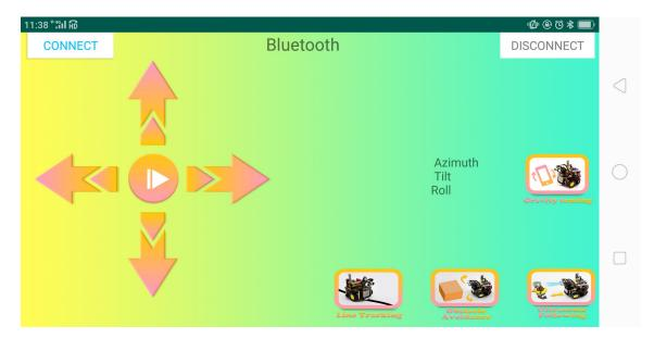
4. After connecting Bluetooth, plug in power and LED indicator of Bluetooth module will flicker. Tap CONNECT to search Bluetooth.
