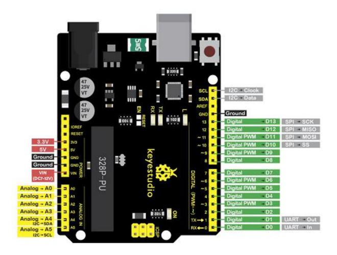
It contains everything needed to support the microcontroller; simply connect it to a computer with a USB cable or power it via an external DC power jack (DC 7-12V) or via female headers Vin/ GND(DC 7-12V) to get started.
