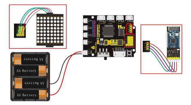
Insert a Bluetooth module, LED indicator of Bluetooth module will flash.
