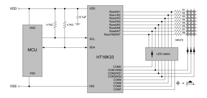
We design the drive module of 8\*8 dot matrix based on the above principle. We could control the dot matrix by I2C communication and two pins of microcontroller, according to the above diagram.
