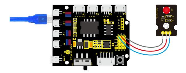
The expansion board is stacked on development board, -, "+" and S pins of LED module are respectively connected to G, 5V and D3 pins of shield.
