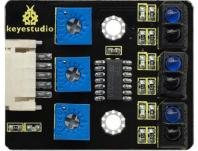
The tracking sensor is actually an infrared sensor.
