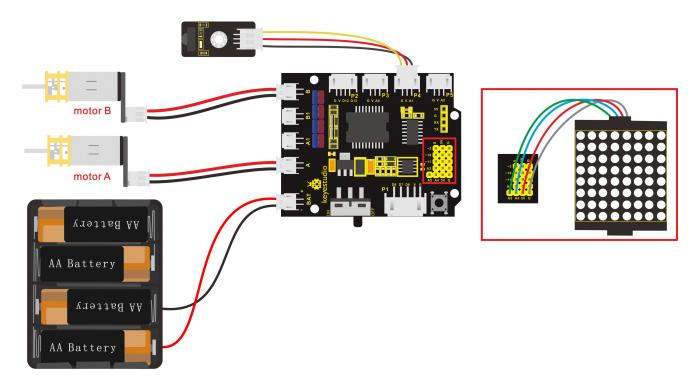
Note: IR receiver is connected to P4 interface.
