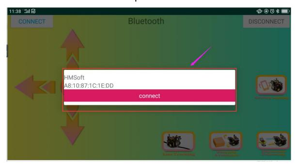
(4) Click "connect" below HMSoft, then the Bluetooth will be connected and its LED indicator will stay on.
