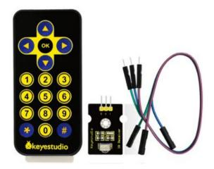
There is no doubt that infrared remote control is ubiquitous in daily life. It is used to control various household appliances, such as TVs, stereos, video recorders and satellite signal receivers. Infrared remote control is composed of infrared transmitting and infrared receiving systems, that is, an infrared remote control and infrared receiving module and a single-chip microcomputer capable of decoding.
