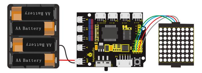
Note: The pin G, V, SDA and SCL of dot matrix module are separately connected to G, 5V, A4 and A5 of motor drive shield. Plug power to BAT
