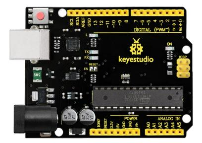
Keyestudio V4.0 development board is an Arduino uno -compatible board, which is based on ATmega328P MCU, and with a cp2102 Chip as a UART-to-USB converter.
