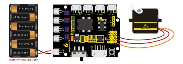
Wiring note: the brown line of servo is linked with Gnd(G), the red line is connected to 5v(V) and orange line is attached to digital 10.
