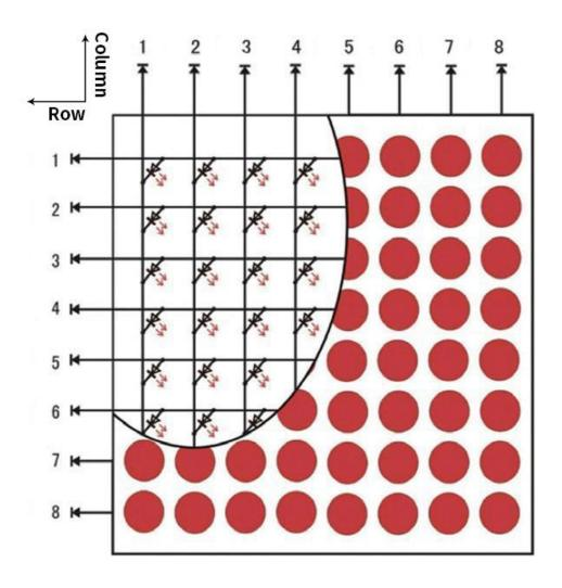
Every LED is installed on the cross point of row line and column line. When the voltage on some line increases, and the voltage on some column line is reduced, the LED on the cross point will light up. 8×8 dot matrix has 16 pins. Put the silk-screened side down and the anticlockwise numbers are 1,8, 9 and 16.
