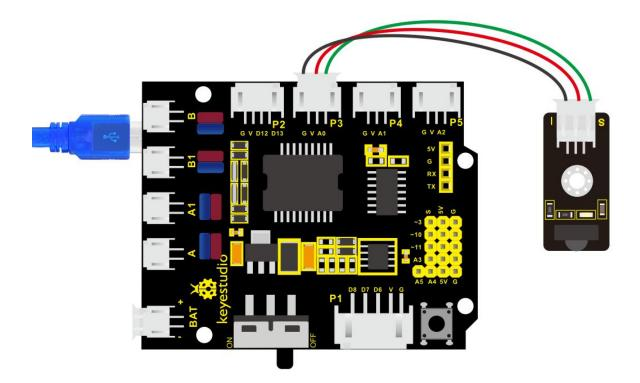
Respectively link "-", "+" and S of IR receiver module with G(GND), V (VCC) and A0 of keyestudio development board.
